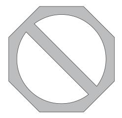
Part A: The outer border with diagonal bar is made from 3 mm thick red acrylic and goes in front of the backboard.
